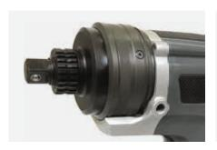
The Dual Speed collar allows the user to quickly shift from high speed rundown to precision torque. The gear shifter has a knurled surface providing a firm grip for ease of shifting. The user can quickly rundown a fastener, then shift to high accuracy torque to bring fasteners to specification, all with one bolting system.
