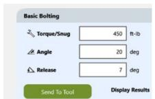
The Connect App provides a simplified graphical interface allowing the user to enter all tool profile, job and administrative setup data on the PC keyboard. Just a single button push and all information is transferred from the PC to the tool saving significant time.
