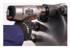
A direct torque measurement system utilizing a strain based transducer in a closed loop monitoring system provides more repeatable torque and enables advanced bolting features.
